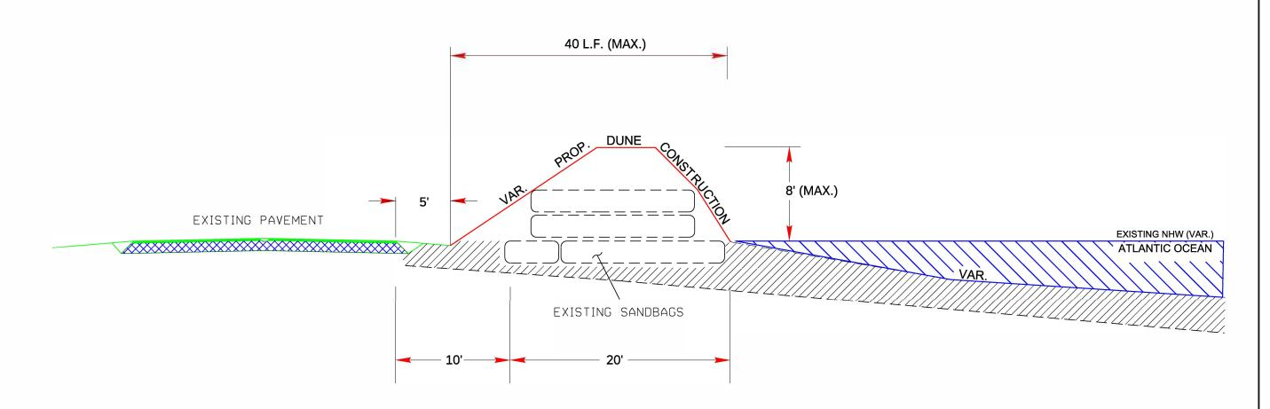
\* MATERIAL USED FOR DUNE CONSTRUCTION SHALL HAVE BEACH QUALITY CHARACTERISTICS AND SHALL BE APPROVED BY THE ENGINEER PRIOR TO PLACEMENT DUNE RECONSTRUCTION: 6,320 L.F.±
